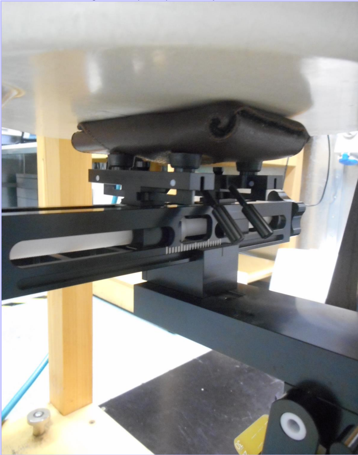
004: Back of EUT Facing Phantom (Case 2) at 5mm Separation
