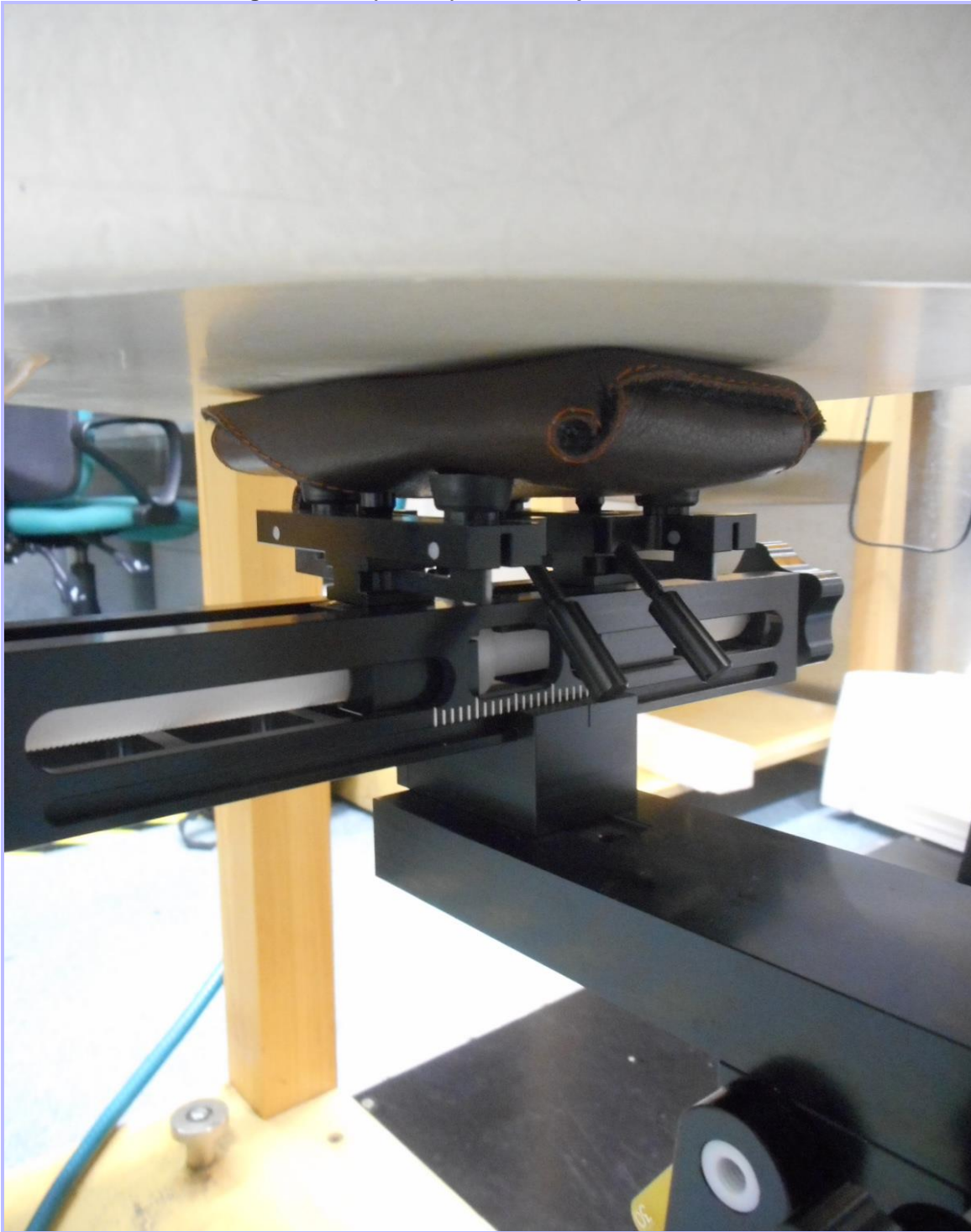
005: Back of EUT Facing Phantom (Case 3) at 5mm Separation
